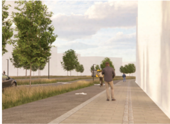
Fig. 108 - View of 30 x 60 tiles with 120cm gap between kerb and guideline
