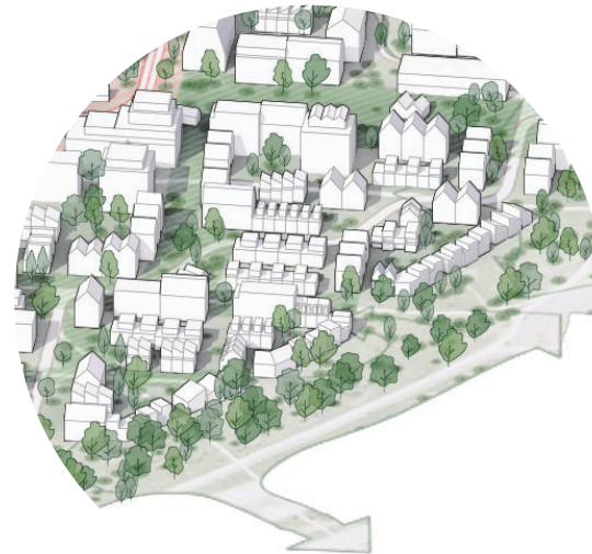
Keldur's southern edge facing Vesturlandsvegur is design to shelter the noise from the motorway and provide comfortable inner courtyards.
