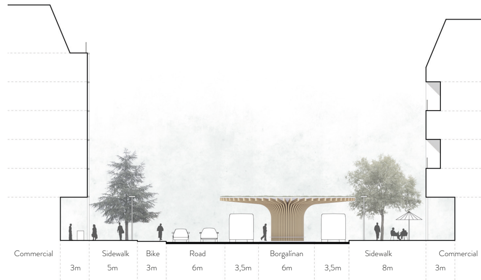
Section BB: Borgalína station - Keldur Center - the second station in the area
