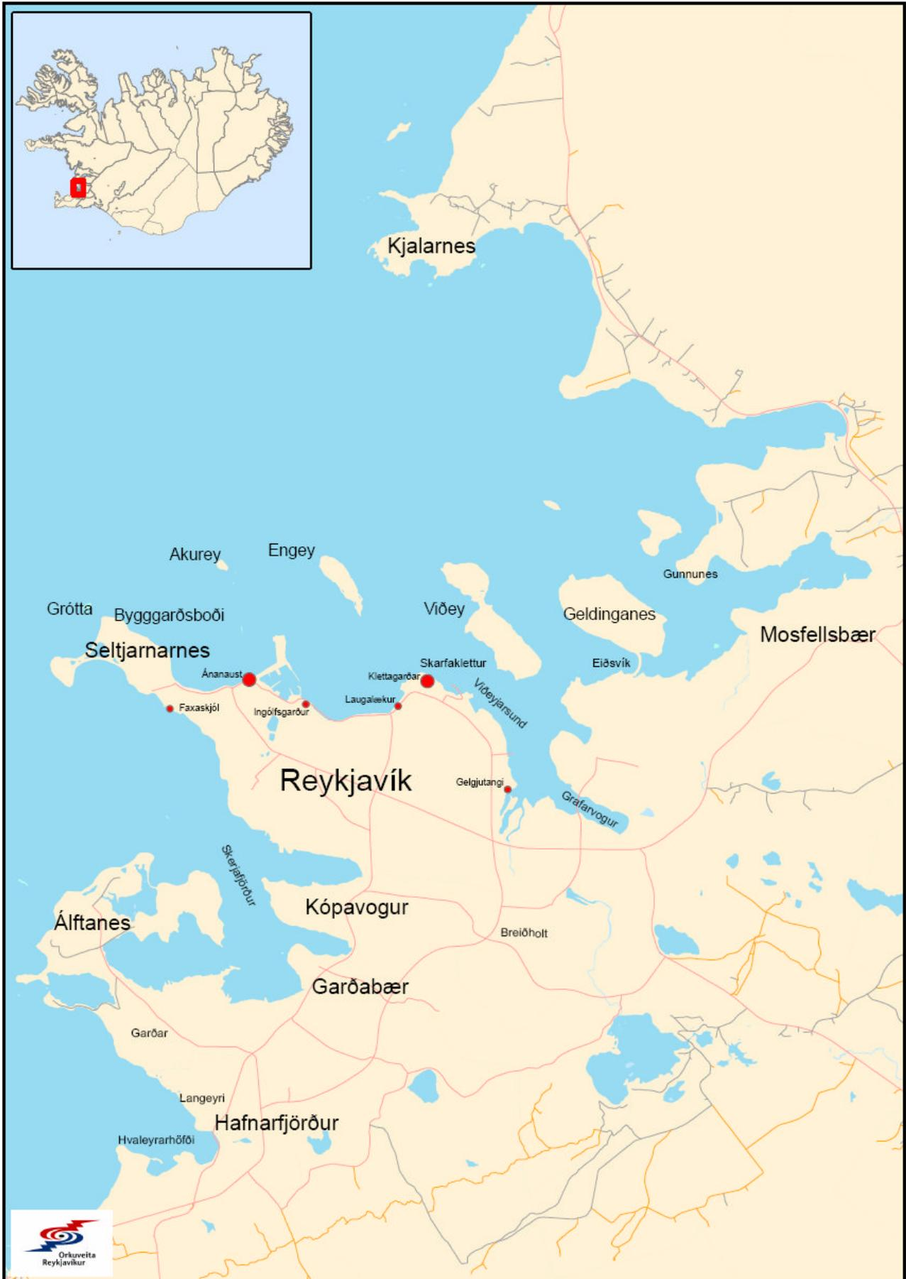
Map 2. Kollafjörður is the bay within Gróttá and Kjalarnes. Small red dots indicate pump stations while the two larger dots show the STPs at Ánanaust and Klettagarðar.
